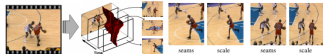
Figure 1: Improved seam carving for video sequences combines the frames of the video to form a 3D cube and finds 3D monotonic and connected manifold seams using graph cuts. The intersection of the manifolds with each frame defines the seams on the frame. The manifolds are found using a new forward-energy criterion that reduces both spatial and temporal artifacts considerably.
